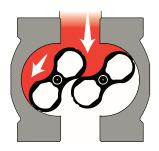
As the left impeller rotates toward the vertical position, gas enters the cavity created between the impeller and the housing.
