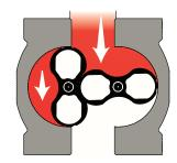
When the left impeller reaches the vertical position, a finite volume of gas is captured in the left cavity.
