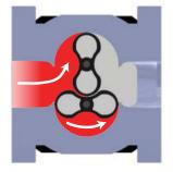
When the bottom impeller reaches the horizontal position, a finite volume of gas is captured in the bottom cavity.
