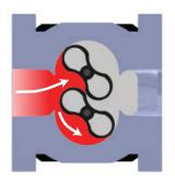
As the bottom impeller rotates toward the horizontal position, gas enters the cavity created between the impeller and the housing.
