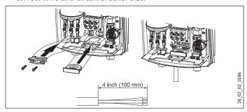
▶ The wire must be fed through the rubber seal located between the hot and cold water connections. Then feed wires through strain relief clamp and tighten clamp down on wire. The "live" wires must be connected to the slots on the terminal block marked L and L. The ground wire must be connected to slot marked with the ground symbol. Strain relief clamp with screws and rubber seal are provided.
