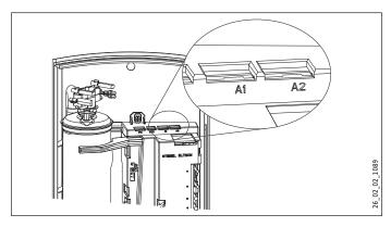
Connect the lead of the electronic temperature control to position "A1" in order to get the maximum outlet temperature of 140 °F (60 °C).
