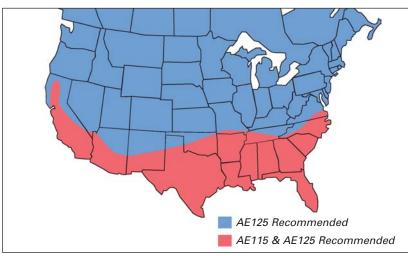
Model AE115 is not recommended in climates where average annual ground water temperature is less than 60°F.
