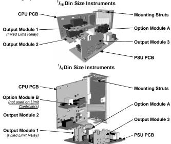
To access module A, first detach the PSU and CPU boards from the front by lifting first the upper, and then lower mounting struts. Gently separate the boards.
