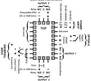
These diagrams show all possible option combinations. The actual connections required depend on the exact model and options fitted.
