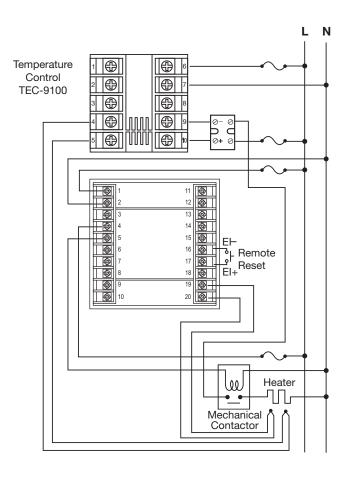
Figure 4.1 Over-Temperature Protection with Remote Reset
