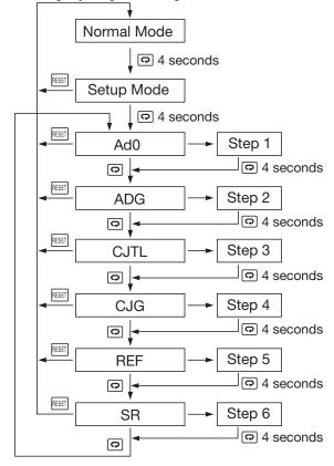
Figure 5.1 Flow Chart for Manual Calibration
