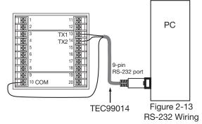
If you use a conventional 9-pin RS-232 cable instead of TEC99014, the cable must be modified according to the following circuit diagram.
