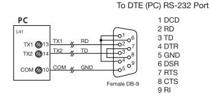
Figure 2.14 Configuration of RS-232 Wiring
