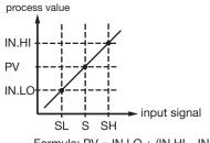
Figure 3.1 Conversion Curve for Linear Type Process Value
