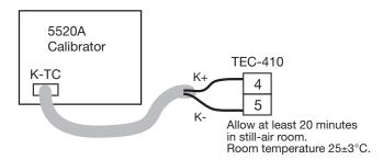
Figure 5.2 Cold Junction Calibration Setup
