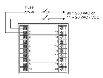
Figure 2.4 Power Supply Connections
