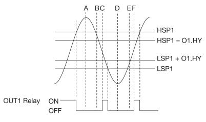
Figure 1.6 A, B, C, D, E, F =Reset is applied O1.HY= Output1 hysteresis
