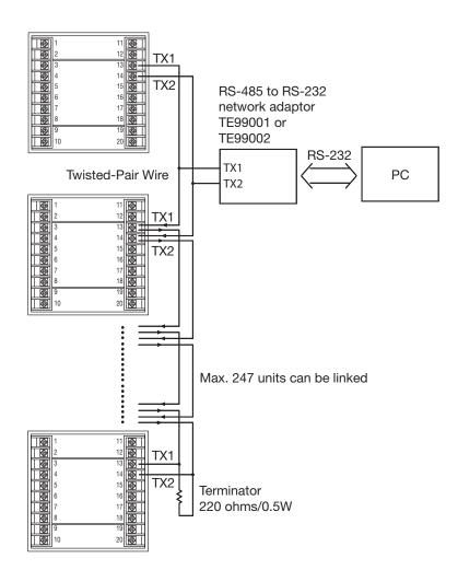
Figure 2.12 RS-485 Wiring
