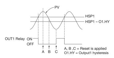
Figure 1.4 High Limit Operation
