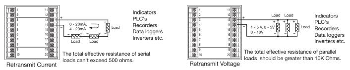
Figure 2.15 Retransmission Wiring
