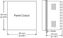
Figure 2.1 Mounting Diagram
