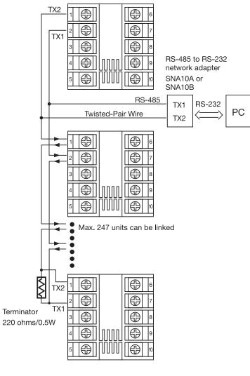
Figure 2.12 RS-485 Wiring
