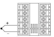
Figure 2.5 Thermocouple Input Wiring
