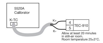
Figure 5.2 Cold Junction Calibration Setup
