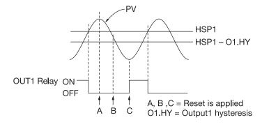
Figure 1.4 High Limit Operation
