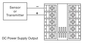
Figure 2.11 Output 2 Wiring
