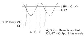
Figure 1.5 Low Limit Operation
