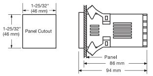
Figure 2.1 Mounting Diagram
