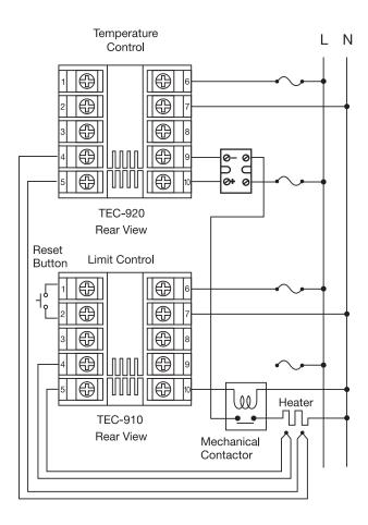
Figure 4.1 Over-Temperature Protection with Remote Reset
