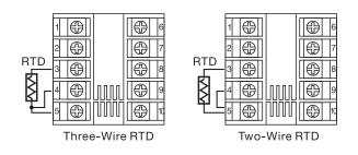
Figure 2.6 RTD Input Wiring
