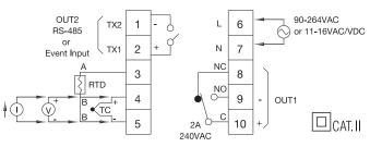
Notes: 50°C max. air ambient Use copper conductors (except on T/C input) ASTM thermocouples (USA), the red colored lead is always negative.
