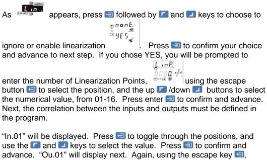
use the and keys to select the value. Press to confirm and advance. "Ou.01" will display next. Again, using the escape key , toggle to the appropriate position. Use the and keys to select the value. Press enter to confirm and advance. Repeat this procedure for each set of Inputs and Outputs, up through a maximum of 16. Press the enter key to confirm. Press to advance to the next program step sequence.
