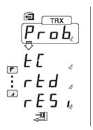
Press . Use . keys to select Range (r1, r2, r3, r4, r5, r6) according to table below and on instruction sheet. Press .
