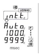
If all zeros "0000" is selected, "Auto" will be displayed and the value will be automatically calculated from 100ms − 999.9 ms. Press to confirm. Press to advance to next program step sequence.
